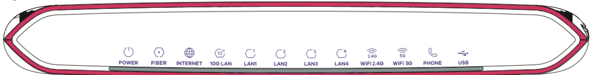
Figure 10 LED Indicators (AX7501-B0 / AX7501-B1)
